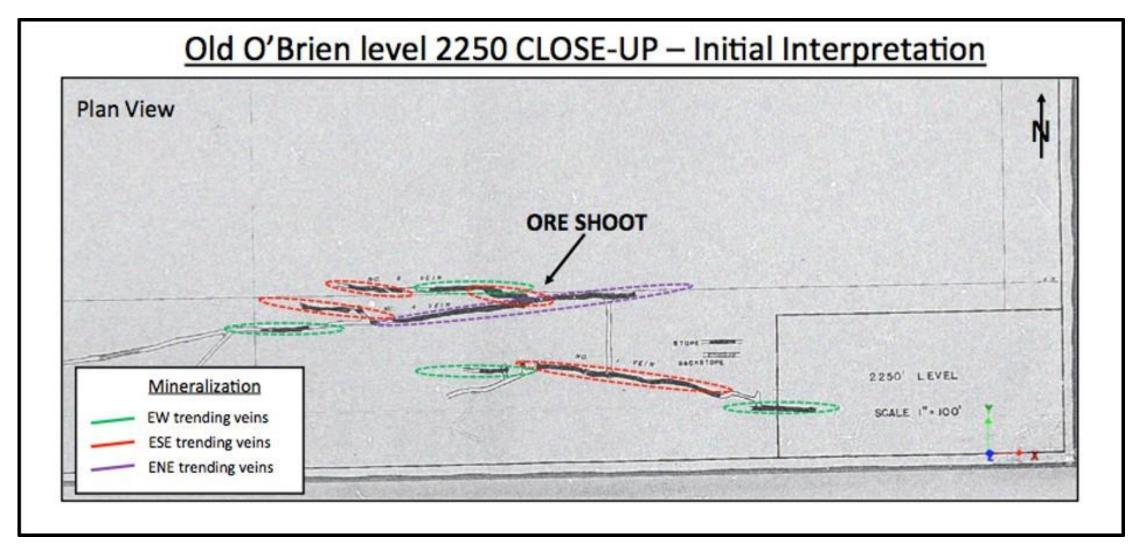
Level plans based on old production data show a strong compatibility between the new model and the geometry of structures previously mined at the O'Brien mine.
