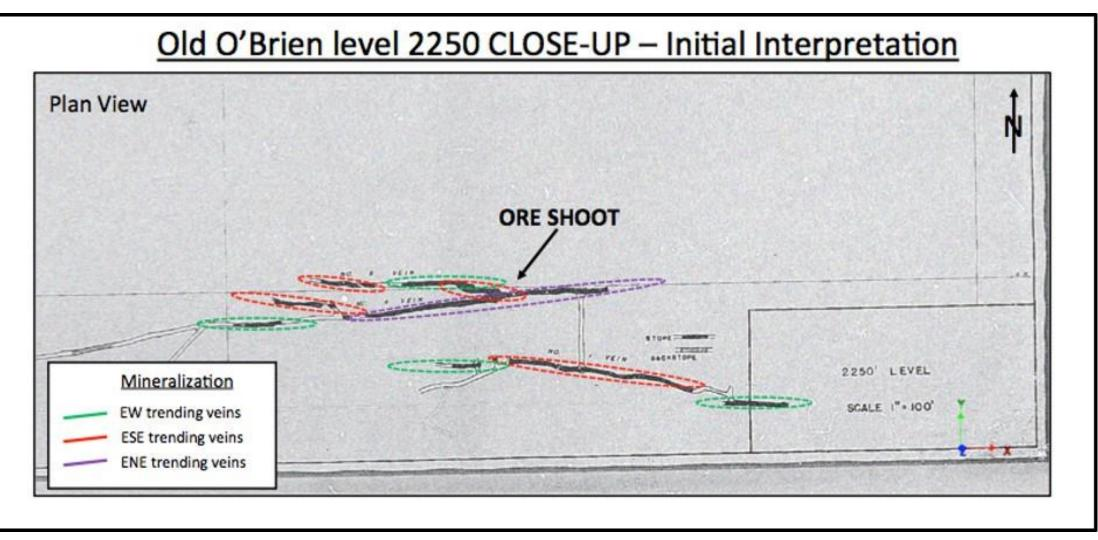
Level plans based on old production data show a strong compatibility between the new model and the geometry of structures previously mined at the O'Brien mine.
