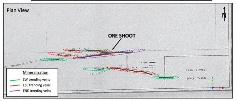
Level plans based on old production data show a strong compatibility between the new model and the geometry of structures previously mined at the O'Brien mine.
